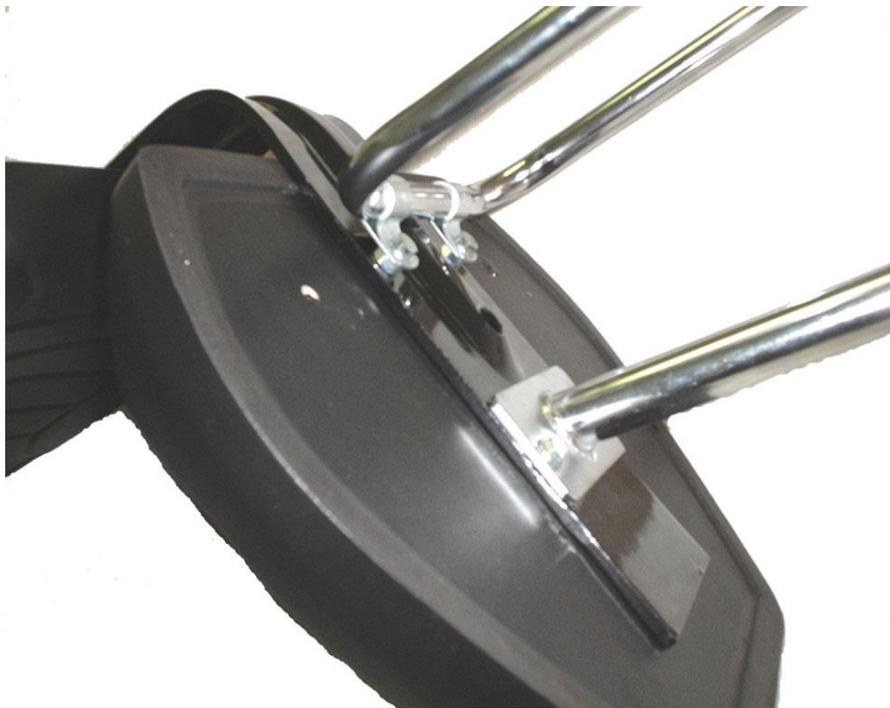
For smaller riders - installing the seat bracket mounting clamps opposite to what is shown in the photo will give additional frame clearance.
