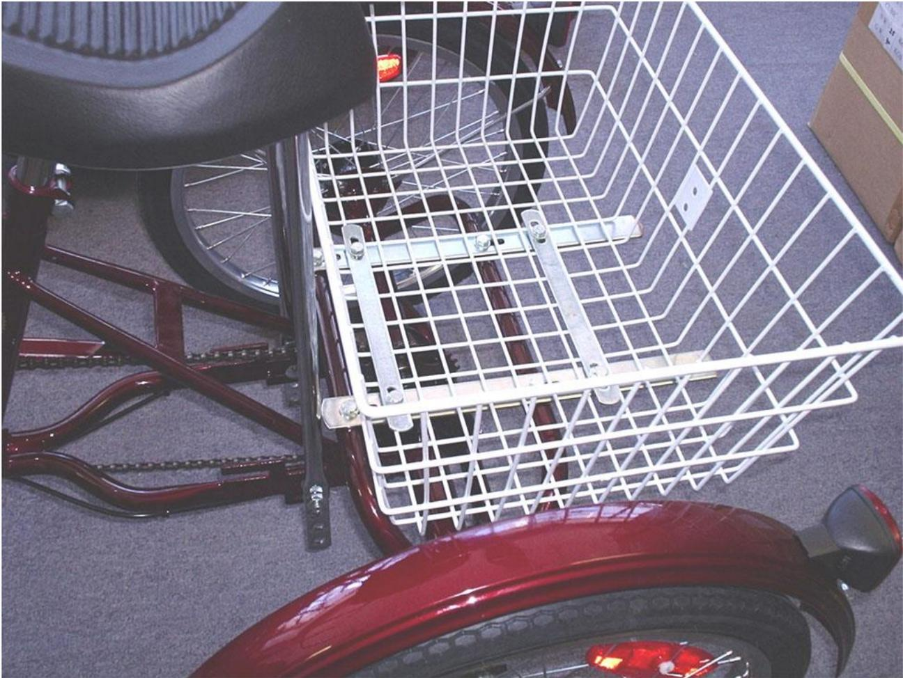
**The secondary basket mounting brackets can be mounted in either direction – across the frame or in the same direction as the main supporting brackets.**
